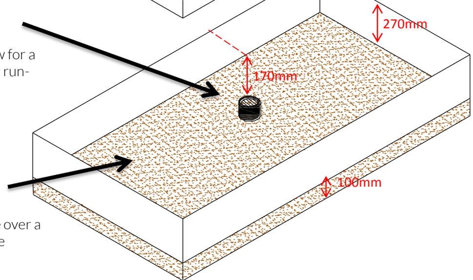
4. Lay a level compacted 100mm granular sub-base over a geo-textile. This will help to spread the load of the concrete installation pad.
