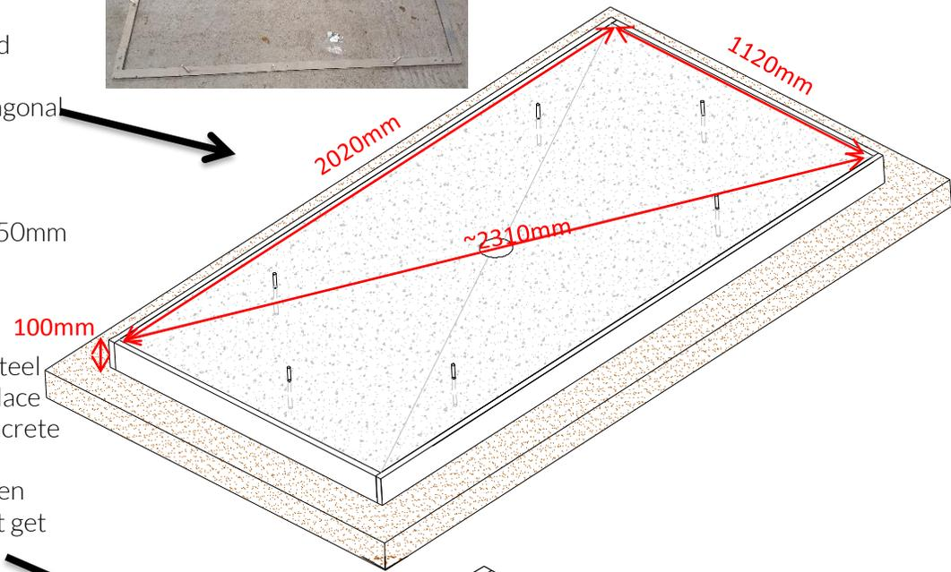
6. Install A142 steel reinforcing mesh (or similar) on 50mm plastic or steel supports or “chairs” to hold mesh vertically centred in shuttering area.
