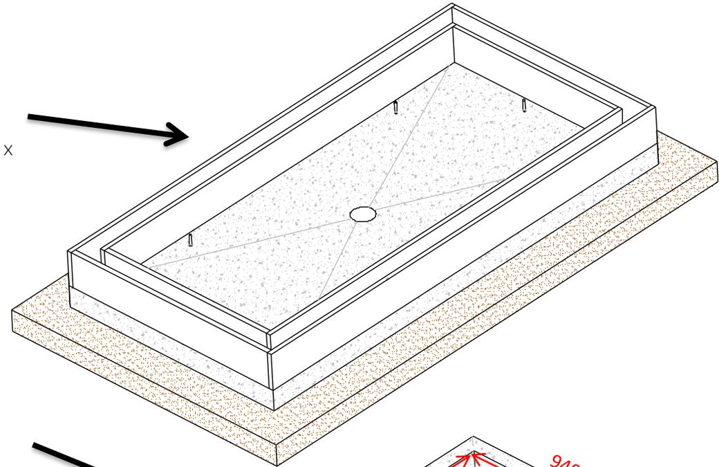
10. Pour concrete between shuttering to cast concrete walls and ensure walls are filled to top of shuttering and level.
