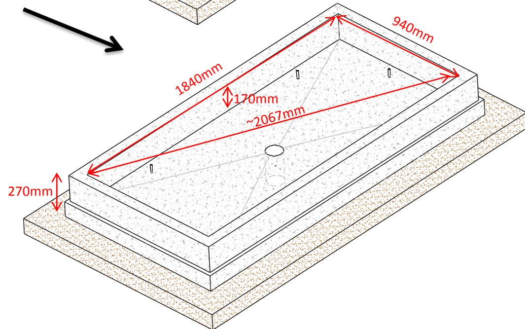
11. Backfill with soil or aggregate around external walls.
